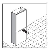
Open the door and push the appliance against the side of the kitchen unit opposite to that of appliance hinges. Fasten the appliance with 4 screws provided in the kit included with the appliance. Snap ventilation grille (C) and hinge cover (D) into position.
